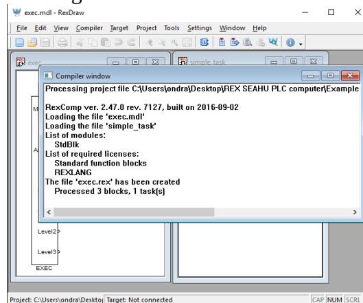
If all is OK , then you can send to module. Menu „Compiler → Compile and Download“ or key F6. After repeatedly compile is view window witch information abut connect to module. In label Target: write IP your module. Default User: admin and default Password: admin .
