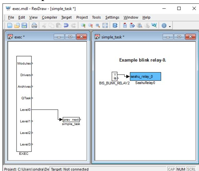
Block “exec” cyclic (here 10x by second) run simple\_task. In simple\_task is inserted block who alternate after 2 sec. generate output on, off who is forward into input of block control relay.
